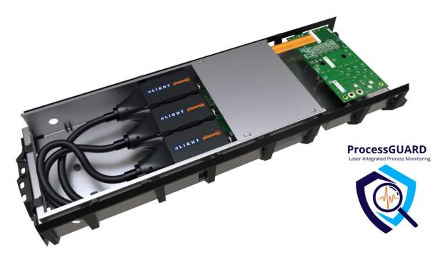
ProcessGUARD integrates the photodiode-based plasmo process**observer** (pso) into the nLIGHT lasers. The process light is captured from the feeding fiber and transferred to pso 6.0 sensors (VIS Sensor 400-1100nm / NIR sensor 750-1800nm / 250kHz sampling rate). The photodiode sensors convert the process light to electrical signals that are evaluated in real time using mathematical algorithms.
